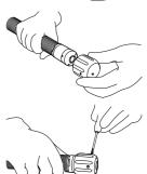
Use the screwdriver to secure the standard skid to the camera head.
