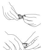
Press the two skid halves together until the tabs lock into the receptacles.
