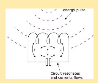
The coil and capacitor are chosen to have a particular resonant frequency.
