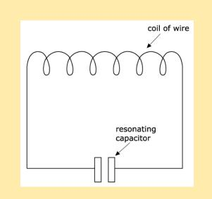
An EMS marker consists of a coil of wire connected in parallel with a resonating capacitor.
