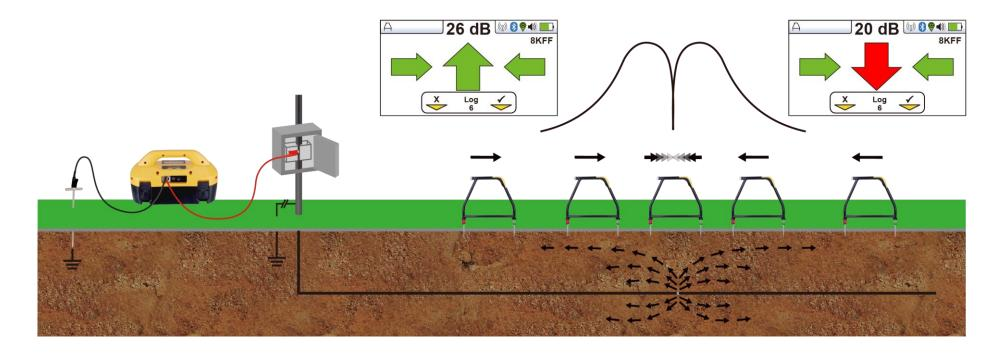
Disconnect all ground connections to encourage the signal to travel through the fault to earth and not a ground somewhere else.
