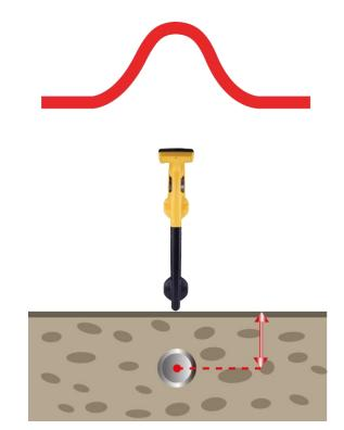
The depth and current readings are continuously displayed on the receiver.
