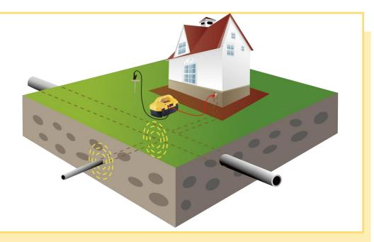
\* Tracing is following the path of the buried line from, or to the transmitter
