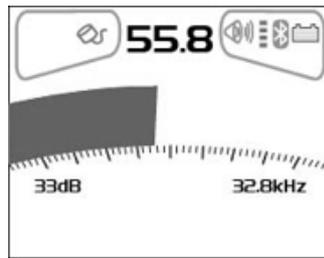
7. Ensure the frequency selected on the vLoc is the same as selected on the transmitter.
