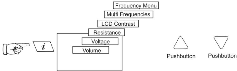
When the “i” (information) pushbutton is pressed, the display will show the audio volume level , use the “+” and “-” pushbuttons to increase/reduce the volume or turn the beeper off (off – low – medium – high).
