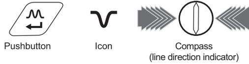
This uses vertical antennas, and provides a minimum or “Null” response over the center of the radiated signal from the buried line. The compass (line direction indicator) shows the direction of the cable (available in Active modes). The color of the compass (line direction indicator) changed from clear to blue when the receiver is in line with the buried line.
