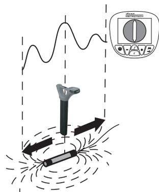
The vLocPro2 receiver must be used in a different orientation when locating a Sonde – due to the way the signal from the Sonde radiates. With the front of the receiver pointing across suspected direction of the Sonde – pinpoint forward and backward (across the Sonde) and then move along the line of the Sonde until the maximum peak is located (in other words rotate the receiver 90 degrees from the orientation normally used when locating pipes and cables).
