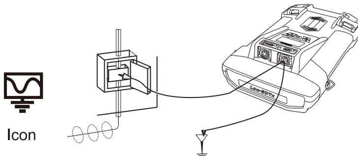
Wherever a direct connection can be safely made without the risk of injury, damage to customer’s plant, or the transmitter, it is the best way of applying the transmitter’s signal.
