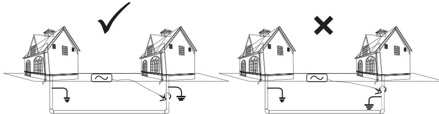
4. If this is not possible to use a transmitter signal clamp, and you have confirmation that the cable is out of service, use a direct connection lead to make an electrical connection to the cable. Removing any cross bonding between cables prevents the signal to travel along commonly bonded cables.
