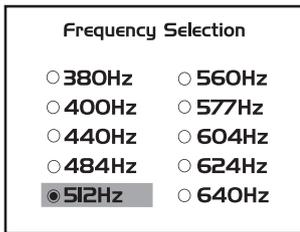
To select the frequencies you wish to use regularly – enter the setup menu by pressing and holding the “i” pushbutton for 2 seconds. Use the “+” and “-” to select the word “Frequency” – then press the “M” pushbutton to display the list of available frequencies.
