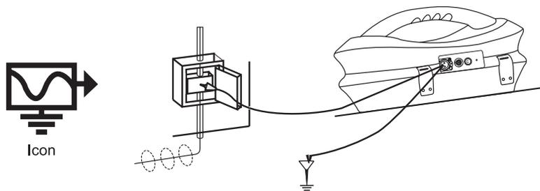
Wherever a direct connection can be safely made without the risk of injury, damage to customer's plant, or the transmitter, it is the best way of applying the transmitter's signal.
