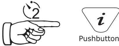
As described previously, a second function performed by the “i” is to access the **setup** menu. Press and hold the “i” pushbutton for two seconds to display the **setup** menu. Use the “+”, “-” to navigate through the various options and use the “M” pushbutton to select. To exit the setup menu, press the “i” pushbutton.
