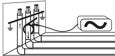
3. When using the signal clamp, both ends of the target cable should be grounded. Apply the clamp below the ground point. Applying the clamp above the ground point will prevent the signal finding the return path through the ground, so is not advised.
