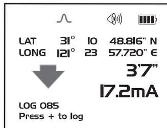
Pressing the “i” (information) pushbutton will display the depth to the center of the radiated signal and a measurement of the current (press the pushbutton briefly – remember if you press and hold – you enter the setup menu. If you do enter the setup menu – press the “i” pushbutton again to return to the locating screen – then try again).
