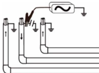
2. Select an SD signal from the transmitter (either SD-USA or SD-EUR).
