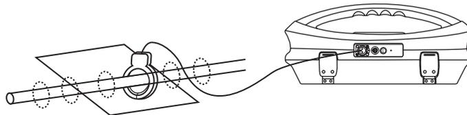
For a clamp to work the current induced by the clamp must flow along the buried line. This means the buried line must have a ground connection at both ends.
