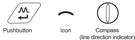
This uses a single horizontal antenna and provides a “Peak” or maximum signal response over the center of the radiated signal from the buried line. The compass (line direction indicator) shows the direction of the cable (available in Active modes). The color of the compass (line direction indicator) changed from clear to blue when the receiver is in line with the buried line.
