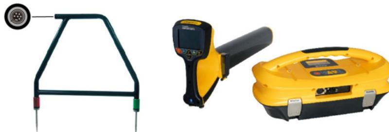
The A-frame accessory is used to detect ground faults on pipes and cables. In the case of pipes, the faults consist of coating defects. In the case of cables, faults are usually caused by insulation damage allowing the metallic sheath (or internal conductor) to become in contact with the ground.
