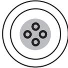
Two pins are used for power in from charger (to charge rechargeable batteries).
