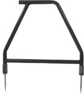
The A-frame accessory is used to detect ground faults on pipes and cables. In the case of pipes, the faults consist of coating defects. In the case of cables, faults are usually caused by insulation damage allowing the metallic sheath (or internal conductor) to become in contact with the ground.
