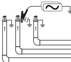
5. **Do not** use the Induction method as the signal will appear on all cables in the area of the transmitter.
