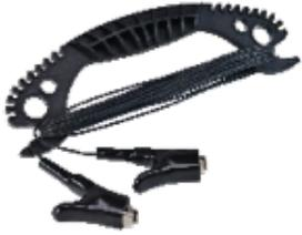
Used to extend the ground connection to a suitable grounding position.
