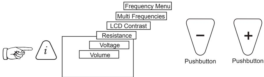
When the “i” (information) pushbutton is pressed, the display will show the volume level of the audio; use the “+” and “-” pushbuttons to increase/reduce the volume or turn the beeper off (off – low – medium – high).
