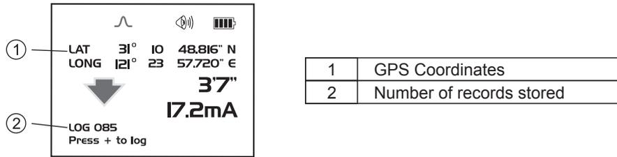
To save a record press the + button whilst in this screen.
