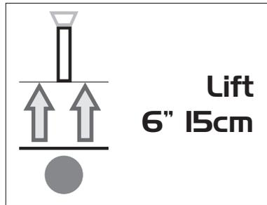
5. Raise the locator 6" (15cm) and again press the “i” button. The depth estimation will be displayed similar as shown below:
