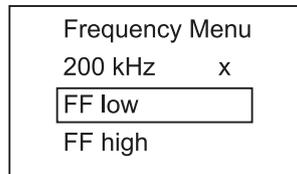
3. Pressing the "+" or "-" pushbuttons, you can scroll up or down through the available frequencies.
