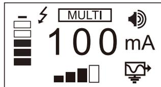
6. The frequencies selected for multi frequency mode will be saved until changes are made even when the multi frequency mode is deactivated.
