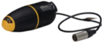
The LPC separation filter (LPC) is used to safely inject a trace tone to a live cable via a domestic mains socket, so that the cable can be traced from the premises to the connection in the street. It is suitable for connecting to voltages between 100V AC and 250V AC.
