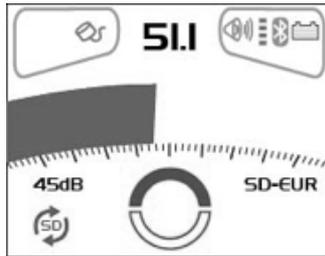
4. If necessary adjust the sensitivity so that the bar graph is on scale. Note that the front half of the circle is red. This indicates that the signal is flowing forwards. If the bottom half is illuminated as below, it will be necessary to perform an SD reset before proceeding. However, if in doubt always perform the reset to be sure the antenna and receiver are synchronised.
