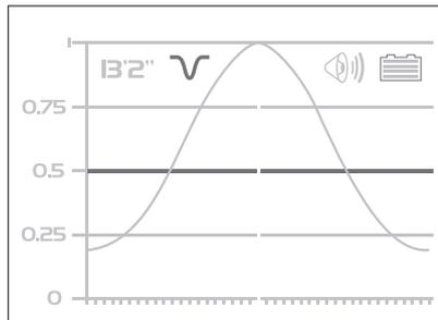
Now slowly move the locator to the side until the line on the graph reaches the 50% line. (or 70% if the 70% rule is used). At this point an audible beep will confirm this position is reached. Mark the ground at this point and then slowly return to the peak position. Continue past this position until the 50% mark is reached on the other side. Mark this position.
