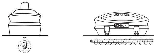
When using the “Induction” mode to apply a signal to a line, ensure that a minimum distance of 50ft (15m) is maintained. This is because the transmitter will transmit signal through the air which will interfere with signals from the cable, resulting in incorrect information.
