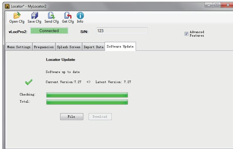
3. If connected to the Web, press the “Get latest sw rev” button. Alternatively, if the software revision required is already saved, use the “File” button to browse to the relevant file.
