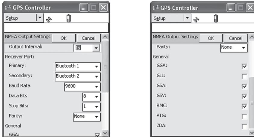
6. Press OK to save parameters to the GPS.
