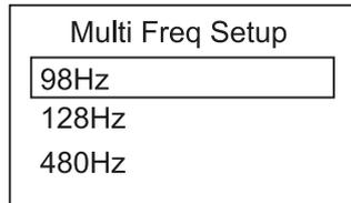
3. Press "f" pushbutton to move the box down and the "+" and "-" pushbuttons to select the second frequency.
