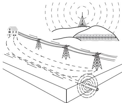
Passive location is used to search an area to see if buried metallic lines are present (known as locating to AVOID). It does not help to identify what buried pipe or cable is present, only to confirm that there is a pipe or cable there. A typical application would be to check an area before installing a fence post.
