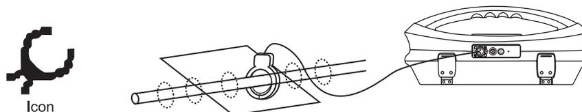
The clamp again is a precise way to apply the locating signal. It is generally used when access to the conductor cannot be achieved to make a direct connection (but there is sufficient access to place the clamp around the cable), or when it is not safe to make a direct connection because the target cable is carrying electricity.
