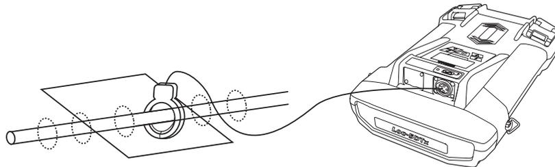
The clamp again is a precise way to apply the locating signal. It is generally used when access to the conductor cannot be achieved to make a direct connection (but there is sufficient access to place the clamp around the cable), or when it is not safe to make a direct connection because the target cable is carrying electricity.
