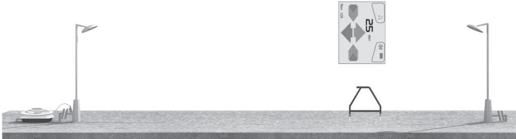
After isolating the line, use the vLocPro2 transmitter resistance measuring function, or a dedicated resistance measuring device to confirm that there is a fault to ground. The A-frame will typically detect faults up to two Mohm and above (depending on the distance from transmitter, soil conditions etc).
