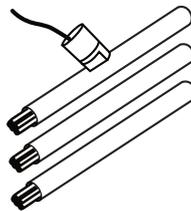
9. The one with the largest reading is likely to be the target cable.
