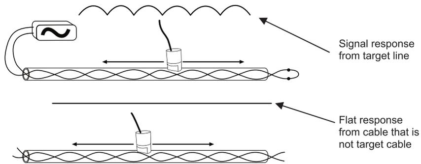
3. At the point of interest, run the remote stethoscope antenna along the suspected target cable. If the correct cable is being assessed the signal will increase and decrease in sympathy with the twist of the two conductors within the cable.
