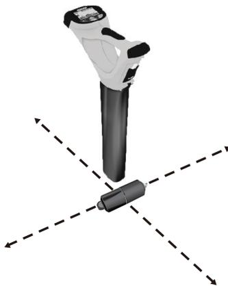
When over the peak position, the depth is automatically displayed. Press the “i” pushbutton to get a more precise depth reading.
