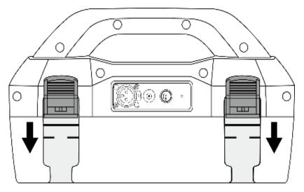
Slide the transmitter onto the tray, it will locate itself in the correct position.
