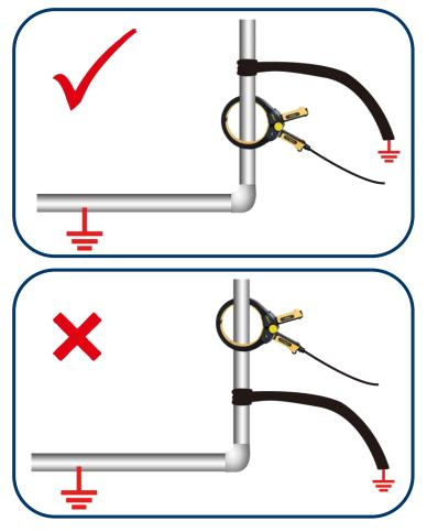
\* Clamps are designed for specific frequencies only, typically 8 kHz – 83 kHz
