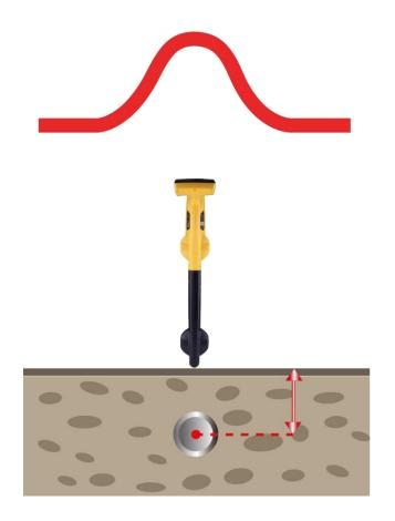
The depth and current readings are continuously displayed on the receiver.
