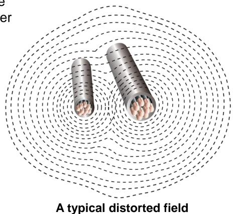
The result is that the locator detects signals from more than one source
