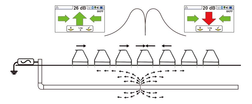
Disconnect any ground connections other than the transmitter ground to encourage the signal to return through the fault
