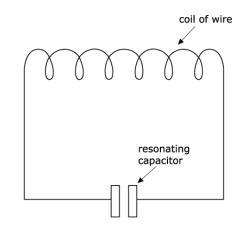
An EMS marker consists of a coil of wire which is connected in parallel with a resonating capacitor.
