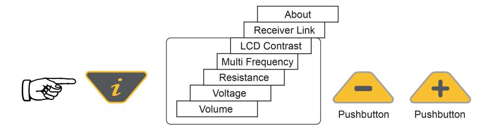
When the "i" (information) pushbutton is pressed, the display will show the volume level of the audio; use the "+" and "-" pushbuttons to increase/reduce the volume or turn the beeper off (off – low – medium – high).
