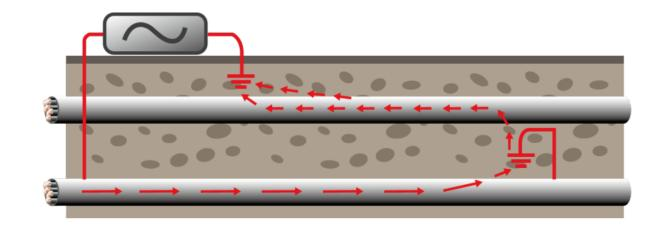
• Signals may use other pipes and cables to return to the transmitter because they represent a lower resistance than the ground.
