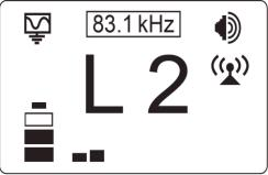
While the icon on the transmitter is flashing, indicating that it is waiting to connect to a receiver, switch on the vLoc3-Pro receiver and enter the user menu by pressing and holding the information button. Scroll down the menu options until Transmitter Link is highlighted.
