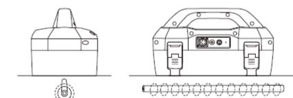
• Induction – induces a signal into a cable or pipe, by placing the transmitter on the surface over the target line
