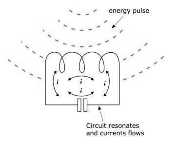
The coil and capacitor are chosen so that they have a particular resonant frequency.
