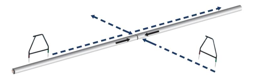
• Repeat the process at 90° to the position of the fault to identify the position laterally. Where the two lines cross is the position of the fault.
