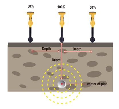
• This distance should be the same as the first measurement taken. If not, it is a clear indication of a distorted or bent field generally caused by signals radiating from adjacent cables.
