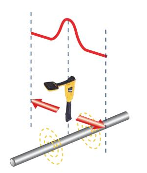
Rotate the receiver until the maximum signal response is shown
