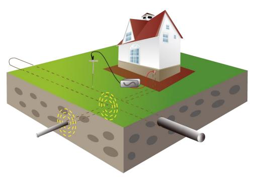
\* Tracing is following the path of the buried line from, or to the transmitter
