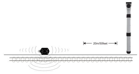
Also note that the signal will radiate out to the side of the transmitter as well as below. For this reason, it is recommended that when applying a signal using the induction method, a distance of at least 20m is kept from the transmitter when pinpointing or taking depth readings. Locating closer than 20m is possible but the operator should be aware that the signal directly received from the transmitter may be strong enough to influence the results.
