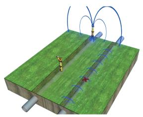
3 The signal should now only be visible in the wanted service but not on the unwanted service. Note that only one service at a time can be nulled out using this method, so if there are more than two services the above may need to be repeated to null out other services.
