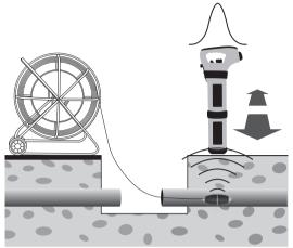
6. Finally check that the vScan is in line with the Sonde by rotating it on its axis to obtain a peak signal. The vScan is now over the Sonde and in line with it.
