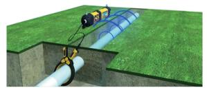
In many situations it is not possible to gain access to a cable for making an electrical contact. Or if there is, it is not safe to do so. The signal clamp provides an efficient and safe method of applying a locate signal to a cable.
