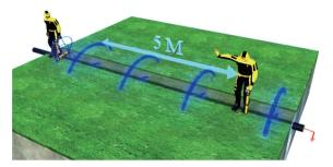
Stand at least 5m apart holding the equipment as below, i.e. with the transmitter and receiver in line with the direction of walking.
