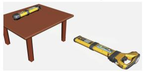
2. Switch on the transmitter and set the output to low. Set the receiver to 33 kHz Sonde mode. Set the sensitivity control so that the largest notch is pointing directly at the mode switch as below.
