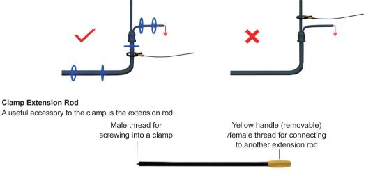
The extension rod is fitted with a 10mm threaded male stud. This male thread screws into the handle of the signal clamp to extend the distance of the clamp. This is very helpful for use in areas with difficult access such as in manholes or overhead cables. (Not to be used on uninsulated overhead power cables.)
