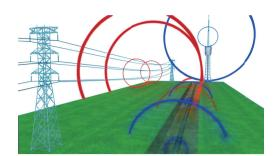
Radio signals are created by low frequency radio transmitters. These are used for broadcasting and communications. They are positioned throughout the world. As the frequencies are very low the signals tend to penetrate and hug the curvature of the earth. When the signals cross a long conductor such as a pipe or cable, the signals are re-radiated. It is these re-radiated signals that can be detected by the Radio mode.
