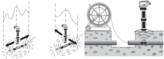
4. Adjust the sensitivity control so that the bar graph reads approximately 75%. Now move the vScan forward and back to detect the largest signal. You will also notice that there will be a "ghost signal" in front and behind the Sonde. This is normal and characteristic of locating Sondes.
