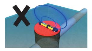
When using the induction mode, avoid placing the transmitter over metallic manhole covers as this will severely reduce the effectiveness of the transmitter and in extreme cases cause damage to the transmitter's circuitry.
