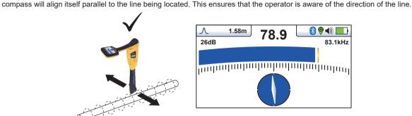
Hold the locator vertically and rotate it on its axis until the compass indicates Forward/Back as above.
