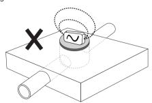
When using the induction mode, avoid placing the transmitter over metallic manhole covers as this will severely reduce the effectiveness of the transmitter and in extreme cases cause damage to the transmitter's circuitry.
