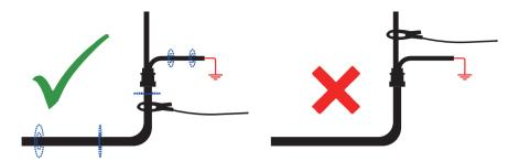
When applying a clamp close to a grounding point where multiple grounds or a grounding bus exists, ensure that you place the clamp around the target line and not to the ground bus/other grounds This will help focus the applied signal to the target line.
