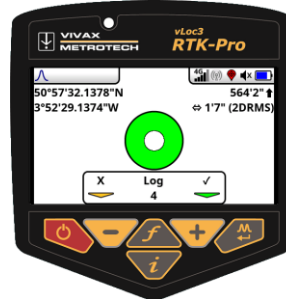
Aligned GNSS Antenna
