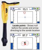
Sonde location - When directly over the sonde the sonde icon appears and depth is shown in upper left
