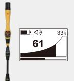
**VM-540** – The VM-540 Sonde Locator comes standard with sonde/camera frequencies of 33kHz, 512Hz, and 640Hz. The VM-540 sonde locator is equipped with a "Passive" Power Mode which will detect the presence of some power lines, and some metallic pipes which radiate 60 Hz from nearby or overhead power lines. Push-button depth displays your depth of cover in feet and inches or metric.
