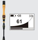
**VM-540** – The VM-540 Sonde Locator comes standard with sonde/camera frequencies of 33kHz, 512Hz, and 640Hz. The VM-540 sonde locator is equipped with a "Passive" Power Mode which will detect the presence of some power lines, and some metallic pipes which radiate 60 Hz from nearby or overhead power lines. Push-button depth displays your depth of cover in feet and inches or metric.
