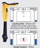
**vLoc3-Cam** – The vLoc3-Cam is the easiest to use sonde locator on the market today. The omnidirectional antenna array allows for approaching the sonde from any position. The directional arrows will guide the user first to the front or rear locate point and then directly to the sondes position.
