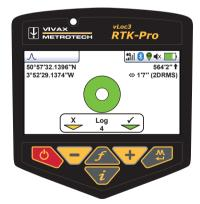
Aligned GNSS Antenna
