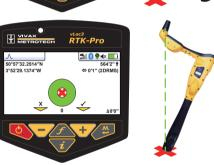
Use the + key to log the Walk Back as complete. This records how accurately the Walk Back was performed and marks the Walk Back as complete in the VMMap Cloud.
