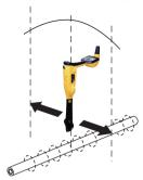
A single horizontal antenna provides a "Peak" or maximum signal response over the buried line.
