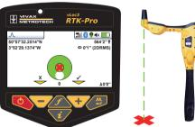
7. As you tilt the locator to get the GNSS antenna over the locator's foot, you aim to get the spirit level bubble into the center of the spirit level. When you have the locator's foot on the ground, and the Walk Back point the red cross and the spirit level bubble will be in the center of the spirit level, as shown in the illustration to the right.
