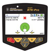
As you walk toward the Walk Back point, you aim to get the red cross in the center of the spirit level. Now the GNSS antenna is over the Walk Back point.
