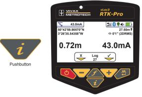
When in a Locate screen, a quick press of the "i" (information) pushbutton will display the depth and signal current.
