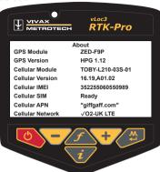
There may be a message "Cellular Module searching" shown for a few seconds. This is normal, as the module takes a few seconds to boot up. The two critical items in the about screen are:
