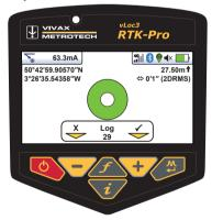
If a valid GNSS/RTK fix is available, an additional screen will be shown with a spirit level. The function of this is described in the "Datalogging" section.
