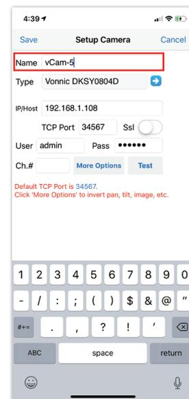
8. For **"Type"** use the blue arrow to the right of the field to view the drop-down list. Select Vivax-Metrotech vCam-5 or Vonnlic and then model DKSY04D in the drop-down list. Now select **"Back"** in the upper left corner to continue.
