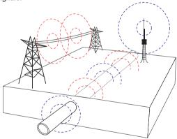
**Radio signals** are created by low frequency radio transmitters. These are used for broadcasting and communications. They are positioned throughout the world. As the frequencies are very low the signals tend to penetrate and hug the curvature of the earth. When the signals cross a long conductor such as a pipe or cable, the signals are re-radiated. It is these re-radiated signals that can be detected by the Radio mode.
