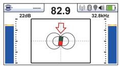
11. Note that when directly over the sonde, it may be necessary to confirm the position of the sonde, left to right. To do this move the locator left to right to identify the position of the strongest signal as indicated on the bar graph. At this time the depth to the sonde will be displayed at the top of the display.
