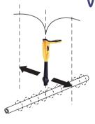
This uses dual vertical antennas. This has the advantage that it provides a sharper response than the "null" mode and is less affected by distorted fields. All other functions are the same as the "Null" mode.
