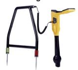
The analogue A-frame accessory is used to detect ground faults on pipes and cables. In the case of pipes, the faults consist of coating defects. In the case of cables, faults are usually caused by insulation damage allowing the metallic sheath (or internal conductor) to become in contact with the ground.
