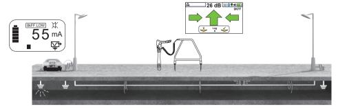
Plug in the A-frame to the receiver accessory socket. When the receiver is switched on, it will automatically default to the A-frame screen
