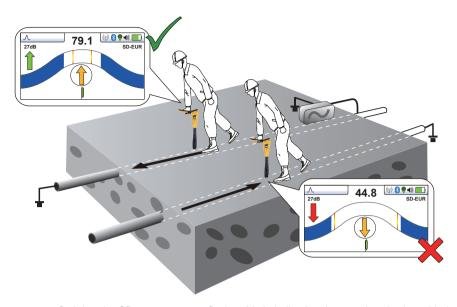
At some point, you may find that the SD arrow starts to flash – this is indicating that synchronization with the transmitter has
