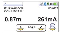
If the GPS function is enabled the GPS coordinates will also be displayed and attached to any saved file. For more information on Data logging and GPS see section 4.2.
