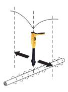
This uses vertical antennas, and provides a minimum or "Null" response over the center of the buried line.
