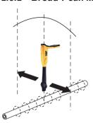
This uses a single horizontal antenna and provides a "Peak" or maximum signal response over the center of the buried line. The compass (line direction indicator) aligns itself parallel to the direction of the cable together with a line position indicator showing which side of the line the locator is (available in Active modes).
