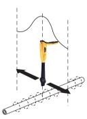
Two horizontal antennas provide a "Peak" or maximum signal response over the center of the buried line. The compass (line direction indicator) aligns itself parallel to the direction of the cable together with a line position indicator showing which side of the line the locator is (available in Active modes).
