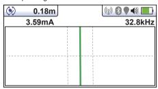
"Tram" lines either side of the line indicate an area of confidence. The closer the tram lines are together the greater the confidence.
