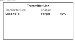
The "Beacon" icon on the transmitter should not be flashing anymore at this point. A solid icon indicates that the link has been established.
