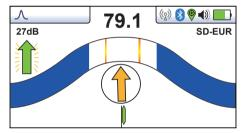
• Re-trace your line back to a point where a solid signal direction is obtained. Precisely pinpoint the line and stand with your back to the direction of the transmitter as you did when you initiated the original sync, and press the "i" pushbutton then the enter/return pushbutton to re-sync with the transmitter signal.
