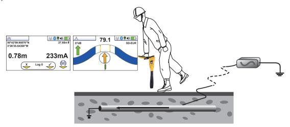
Proceed to locate, trace, pinpoint as required ensuring at all times the green forward arrow is illuminated. If at any time the
