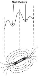
Because of this construction, the Sonde gives a different "Peak" pattern note that there are three distinct peaks – a small peak – a large peak – a small peak with two "Nulls" between the peaks. The Sonde is located under the center of the "large peak".
