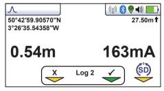
Note that if Omni mode is selected the orientation of the locator is not important but it is still necessary to pinpoint the line accurately before taking a depth measurement.
