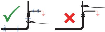
When applying a clamp close to a grounding point where multiple grounds or a grounding bus exists, ensure that you place the clamp around the target line and not to the ground bus/other grounds. This will help focus the applied signal to the target line.
