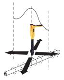
When you see the two double ended arrows around an icon, this means that the line is detectable regardless of locator blade orientation. It is very useful for quickly checking an area for buried lines using a grid search as one sweep will catch all locatable lines. In the classic screen the Omni feature is available in the "Peak" and "Broad Peak" modes.
