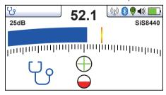
4. If necessary, adjust the sensitivity so that the bar graph is on scale. Note that the front half of the circle is red indicating slight signal distortion, and the polarity sign is "+". This indicates that the signal is flowing forwards.
