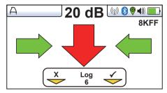
To record data press the "+" button. The soft key on the display will momentarily go green indicating that the data is stored, and the Log number will increment.
