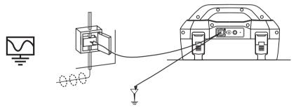
Wherever a direct connection can be safely made without the risk of injury, damage to customer's plant, or the transmitter, it is the best way of applying the transmitter's signal.
