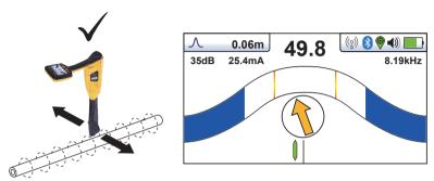
Hold the locator vertically and rotate it on its axis until the compass indicates forward/back as above.
