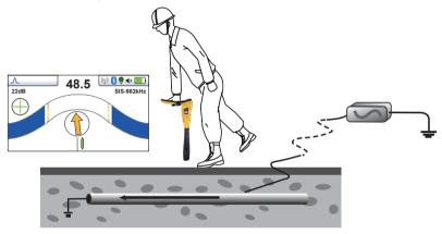
Locate the line as previously described. The "+" "-" indicator and the line direction indicator will show "+" and forward when the correct line is detected.
