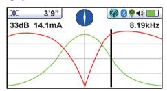
To take a plot first locate the target using one of the other locate screens. Now select the Transverse Screen by a prolonged press of the return button. Repeat this until the Transverse screen appears.
