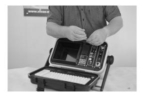
• Use the small handle at the top of the module to carefully slide out the module.
