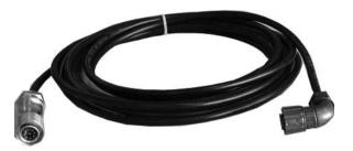
This cable is to connect the command module with cable reel. The 90 deg plug fits to the cable reel (and is normally left connected). The straight plug fits the socket on the control module, and is locked in place by the knurled locking collar. Pull on collar when connecting and removing the plug from the socket.
