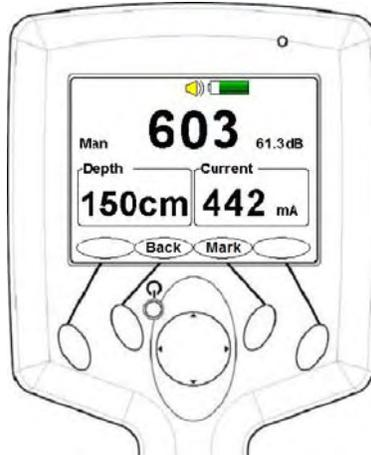
Figure 1-11 Data Logging Depth Measurement Interface
