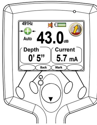
Figure 2-4 Depth & Current Measurement Screen
