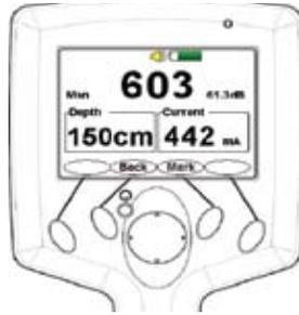
Figure 5-10 Data Logging Depth Measurement Interface
