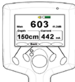
Figure 5-9 Depth Measurement Interface
