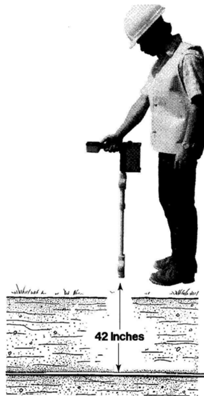
Figure 4-7: Determining the Depth of a Conductor
