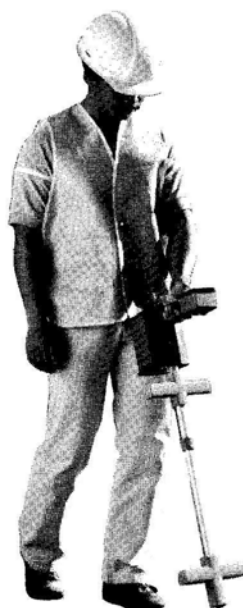
Figure 4-5: Position of Receiver for Tracing
