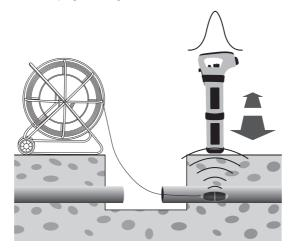
7. Now push the Sonde in a couple of meters and repeat the above to mark the pipe or duct route. Keep the insertion intervals small (2 to 3m) to ensure the Sonde is not lost.
