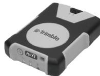
For those wishing to work with accuracies better than 1 meter, the Trimble ProXT/XH provides a simple and cost effective solution. The ProXT operates in a very similar way to the Holux in that it has two LEDs indicating that there is Bluetooth lock and another for GPS lock. Bluetooth pairing is one in the same way as the Holux described above. Data gathering is exactly the same as with the Holux described above.
