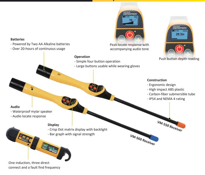
The VM-550 and VM-560 are general-purpose locators used to detect buried pipe and cable services in various situations.
