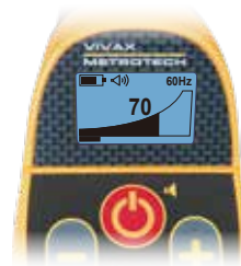
Peak locate response with accompanying audio tone
