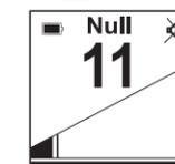
The Null screen shows a minimum signal over the cable. Both the bar graph and numeric value indicate signal strength. The position of the cable is indicated by a minimum signal. This method gives a sharp null over the cable and is useful for tracing the approximate position while walking the route. Caution should be taken though as the null signal can be displaced to the side by a distorted signal.
