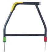
The VM-510FFL+ standalone A-frame is primarily a cable sheath fault finder. The fault must be in contact with the ground to be detectable. It can detect other conductors to ground faults such as pipeline coating defects or cable conductor to ground faults.
