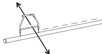
Also the speaker will emit a pulsed tone one side of the cable and a solid tone the other, so it is possible to locate without looking at the screen. If necessary, adjust the volume by using short presses on the **On/Off** button.
