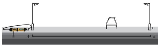
After isolating the line, if available, use the resistance measuring function on the transmitter, or, if not, use a dedicated resistance measuring device to confirm that there is a fault to ground. The A-frame will typically detect faults up to 2 mega ohm (depending on the distance from transmitter, soil conditions, etc.).
