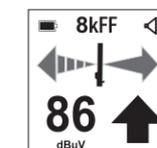
This is the default screen and displays both the cable location and the direction to the fault.
