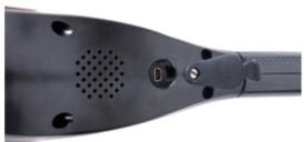
The USB connector is located on the underside of the electronics housing, next to the speaker grill. It is used for software updates.
