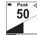
This screen shows a peak level signal. The bar graph and numeric value are both indicating the maximum signal over the cable. The Peak signal is the most accurate signal and should be used to pinpoint the line of the cable if high accuracy is required.
