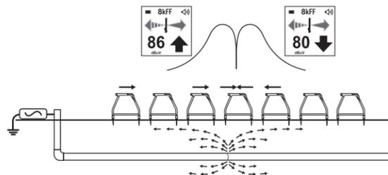
Eventually the A-frame will detect the fault signal and the “Fault Direction Indicator” arrow will point forwards.
