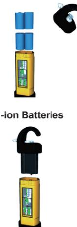
Remove the battery pack by unscrewing the two fasteners of the battery compartment. Align the red dot on the charger with the dot on the charging socket, situated at the base of the battery, and connect together. Connect the charger to the mains and switch on. The charging LED on the charger will illuminate red until the batteries are charged. The LED will then turn green indicating a full charge.
