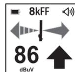
Note that if the spikes are not in the ground or there is only a very small signal, the dB reading and arrow may not be visible. These are only shown when there is a valid fault find signal.
