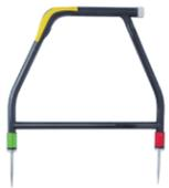
The VM-510FFL+ standalone A-frame is primarily a cable sheath fault finder. The fault must be in contact with the ground to be detectable. It can detect other conductors to ground faults such as pipeline coating defects or cable conductor to ground faults.
