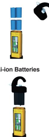
Remove the battery pack by unscrewing the two fasteners of the battery compartment. Align the red dot on the charger with the dot on the charging socket, situated at the base of the battery, and connect together. Connect the charger to the mains and switch on. The charging LED on the charger will illuminate red until the batteries are charged. The LED will then turn green indicating a full charge.
