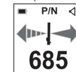
This mode uses the peak and null antenna to indicate the position of the cable on the Left/Right indicator. The numeric value indicates the peak value. In a non-distorted signal field the maximum peak indicator will coincide with the Left/Right indicator null position (i.e. the bar will be centralised). If they do not coincide the signal is distorted and the information should be treated with caution.
