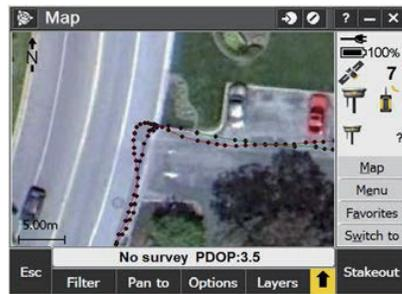
**Spar Hardware** and model-based FieldSens software integrate seamlessly with Trimble GNSS receivers and robotic total stations within an Access-based workflow. Any external GNSS receivers supported by existing Survey Styles can be used in a Spar measurement. Trimble S- and VX-series total stations are supported, as are the controller platforms Trimble TSC3, GeoXR, and Tablet.
