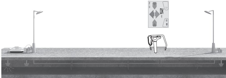
Plug in the analogue A-frame to the receiver accessory socket. When the receiver is switched on, it will automatically default to the A-frame screen.
